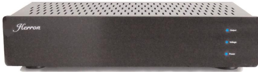
The VTPH-2 features a ½ inch thick anodized aluminum front panel with three lights for monitoring the operational readiness of the unit. When the VTPH-2 is powered up, the automute feature is engaged until the unit is ready for operation. The first indicator on the panel is the Power LED, which indicates the unit has been turned on. After a few moments, the voltage LED gradually brightens, as the voltage to the filaments slowly increases. When the
